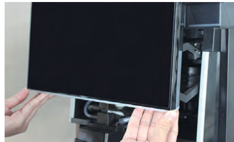
2. Lift the front operation panel
