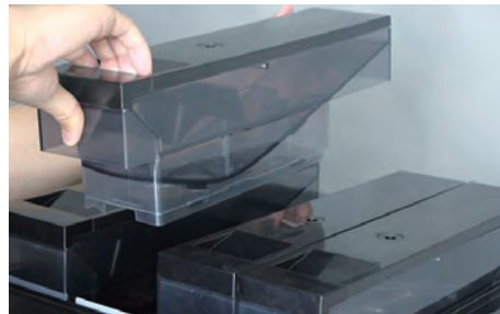
4. Remove bean hopper upwards
