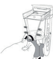
Figure 3: Unscrew the knurled screw retaining the piston stem cover, remove cover
