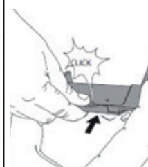
Figure 14: Hook the scraper on its support, insert the support into the lower guides
