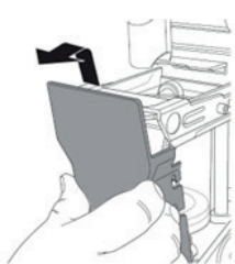
Figure 1: Remove the waste conveyor blue cover
