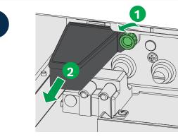
To access the liquid waste conveyor, remove the (liquid and solid) waste trays.
