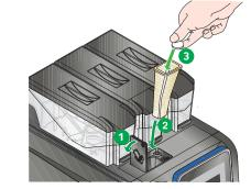
Only use products specifically conceived for coffee machines. The detergent chute is only to be used for washing the brew unit.
