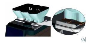
Pull the hopper closing device (a) towards the front of the machine.
