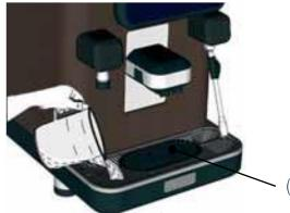
At the end of the working day, pour a jug of hot water into a basin (2) to remove any encrustation in the drain; remove it and wash it with running water.
