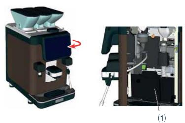
Open the front door panel door and pull out the grounds drawer (1), empty it and wash it under running water.
