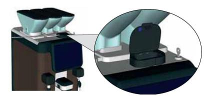
Use a damp sponge to remove any residue in the inside of the door and in the decaf coffee conduit.
