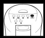
**Step 6:** Now Press the 'HOT WATER' button to begin the FLUSH cycle. The Brewer will start to pump water, and after several seconds, water will be dispensed into the container. The water jet may be seen to 'splutter' for a short while at the start, this is normal.
