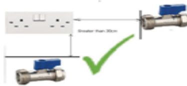
Ideal: Water more than 30cm away from and below socket outlet.
