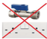
Water above the socket outlet
