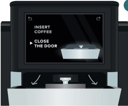
**3** The brewer will open the Freshpack door and the on-screen instructions will ask for the appropriate Freshpack. Once inserted, follow the on-screen instructions. If the incorrect Freshpack is inserted, the brewer will ask whether to continue, see compatible options for the inserted Freshpack, or go back to the home screen.
