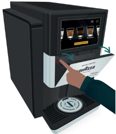
If the brewer is without power, the Freshpack door can still be opened by removing the drip tray and the Freshpack bin, then pressing the red button on the chassis inside the brewer.
